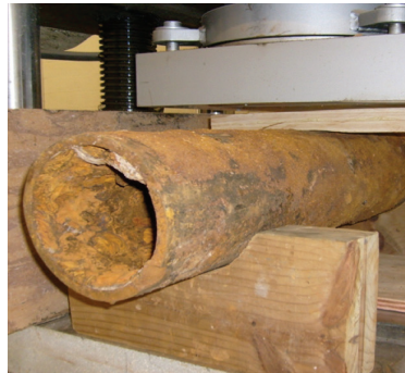
Pipe Sample Being Load Tested
