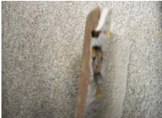
Air inclusion, or air trapped within the wall of the pipe during the manufacturing process, reduces the overall strength of the main and makes it more prone to leaks and breaks. Pit cast mains may have air inclusions.
