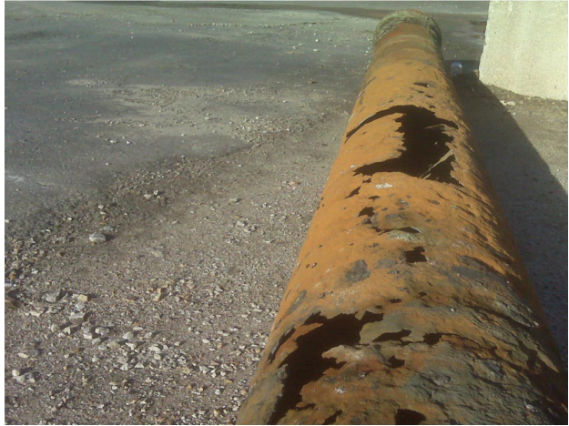
The image above shows a ductile iron pipe that was located along a coastal area in New England. Installed in 1975, the pipe lasted only 30 years.
