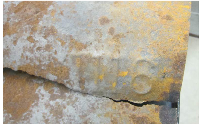
Manufacturers would stamp the pipe with the lot number or year manufactured. This actually becomes a stress point in the main and could result in breaks.
